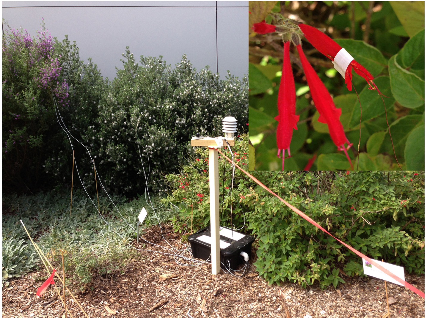
Fig 2. Equipment set up in the field to collect flower temperature readings. Inset shows the TSM sensor attached to a petal surface.
