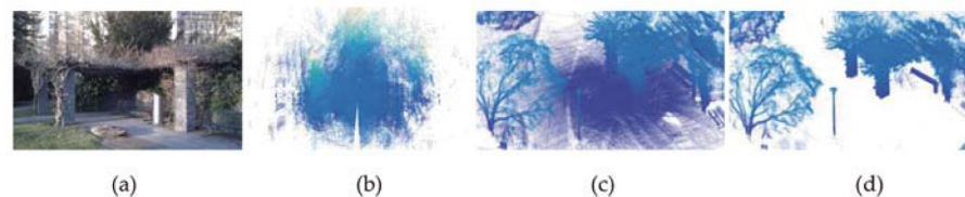
Fig 12. Mapping result of Gazebo data set. (a) Scene image (b) Raw range scans. (c) Mapping result with noises and ground surface. (d) Mapping result without noises and ground surface.
