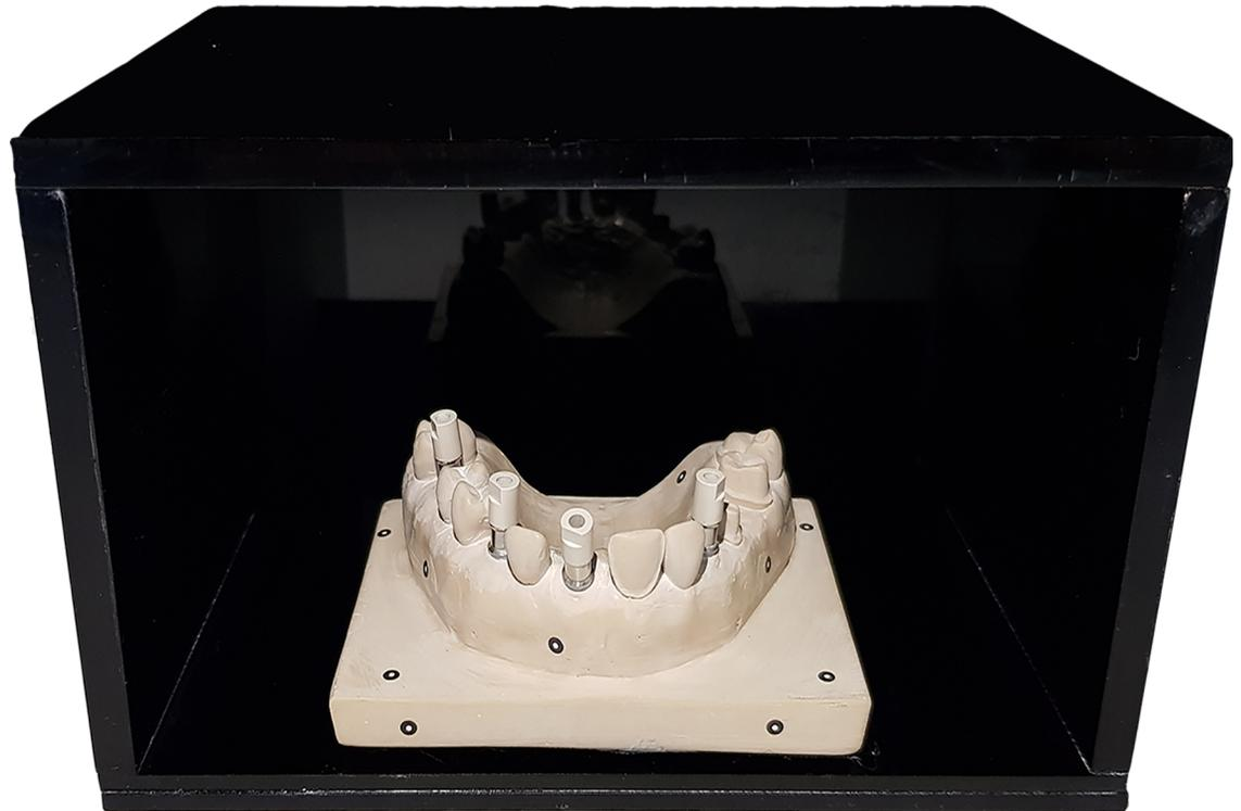
**Fig 1. Master cast inside the methacrylate box to record digital scans.**
