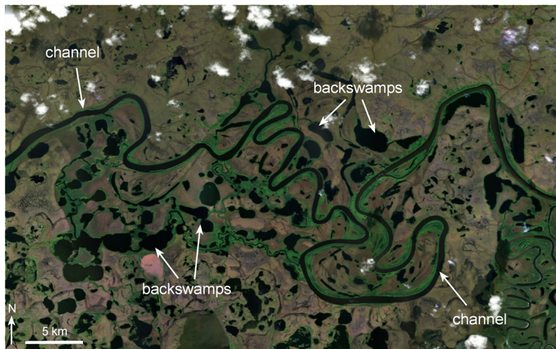
(C) Laterally unconfined, continuous channel, meandering, backswamp sand bed LU_C_Meand_BSw_Sbed
