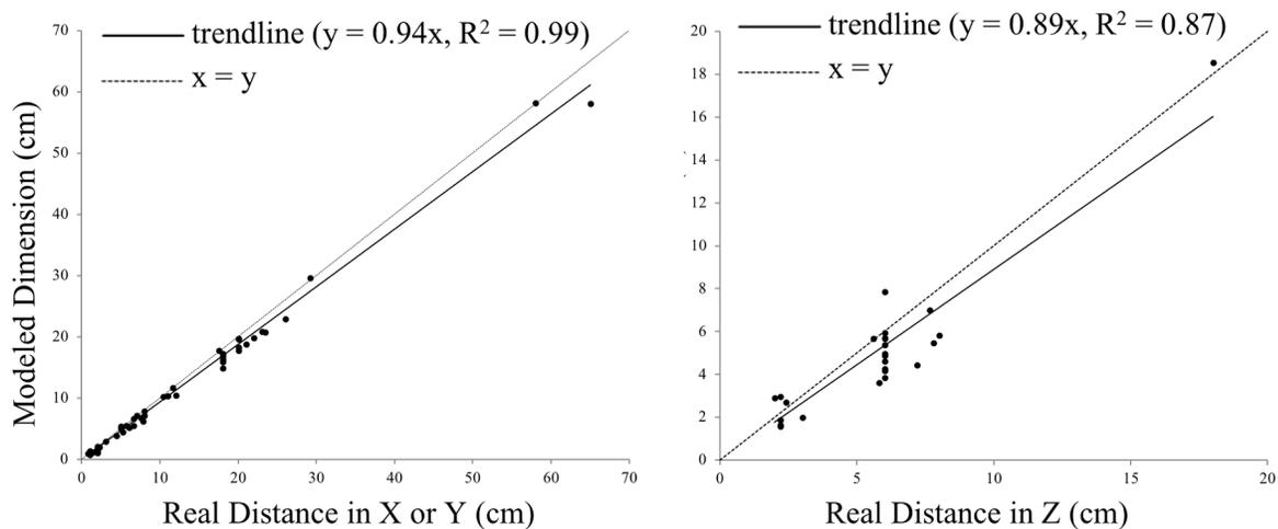
**Fig 6. Accuracy of 3D model in terms of point-to-point distances.** The root mean square errors (RMSE) of our models were 1.48 cm in X-Y and 1.35 cm in Z, with models underestimating dimensions in both X-Y and Z.
