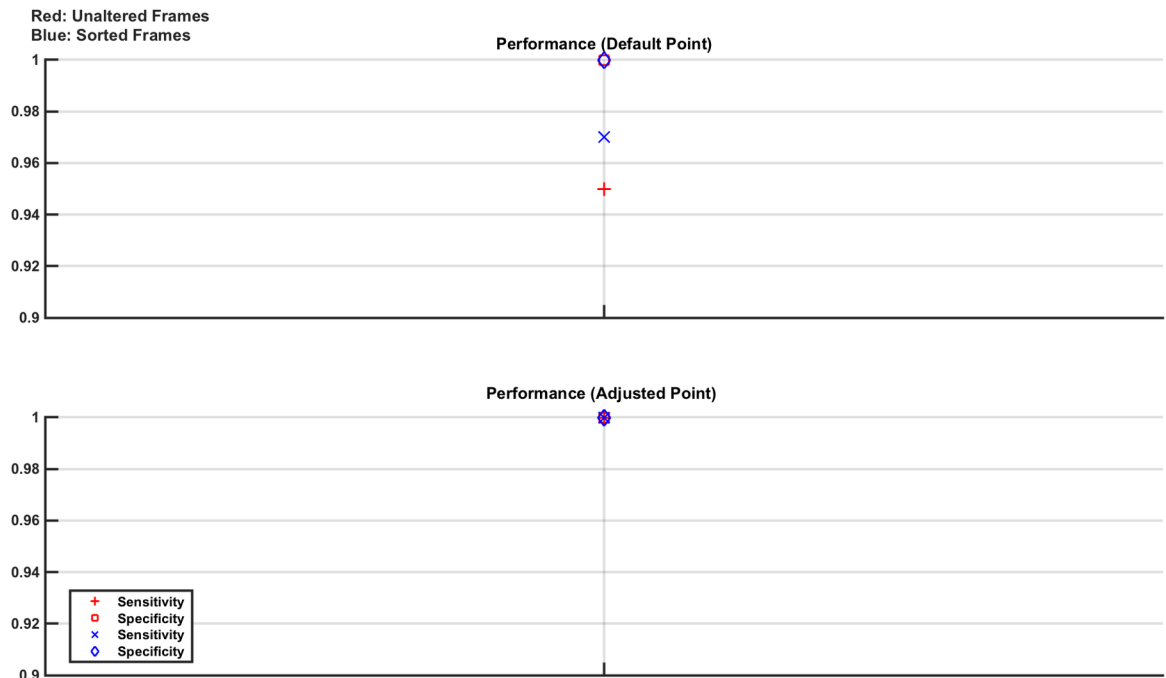
Fig 8. Classifier results from test data in numerical model Study 4: Effect of electrode location. The models are trained using frames from the base numerical model as the normal and eight lesion models produced from the normal and all combinations of the 30 ml or 60 ml lesion at one of the 4 locations. The frames are contaminated with noise at 60 dB SNR. As usual, two classifiers are produced, one trained with unaltered frames and one with sorted frames. These are then tested with the electrode ring placed at one of two possible locations differing from, and parallel to, the original by \pm 2 mm. The results show that classifier performance, though excellent, is noticeably affected by even these small changes in electrode positioning. Using the adjusted operating point however, mitigates against the reduction in sensitivity introduced by the electrode positioning change.
