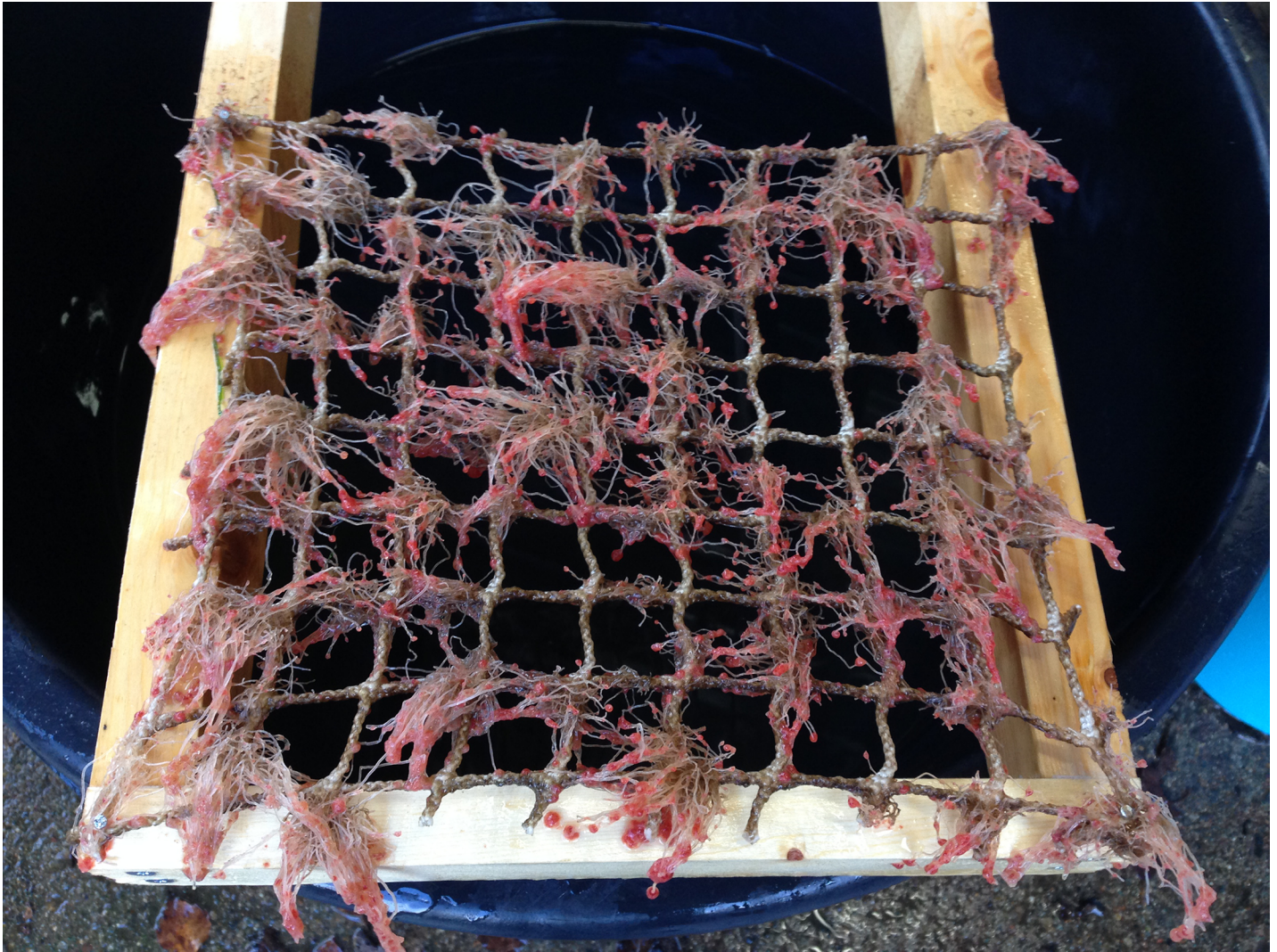
Fig 2. Hydroids on net sample attached to a frame for high-pressure cleaning.
