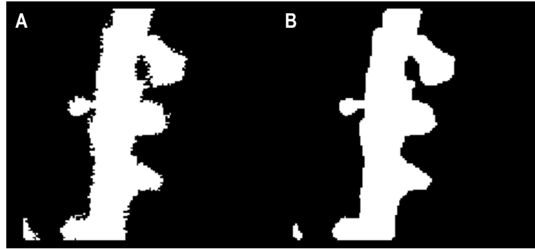
Fig 3. Surface smoothing of binary image. (A) Initial binary image contains a significant noise around its perimeter. (B) Surface-smoothed image lacks kinks, as well as spurious or diagonally-connected pixels.
