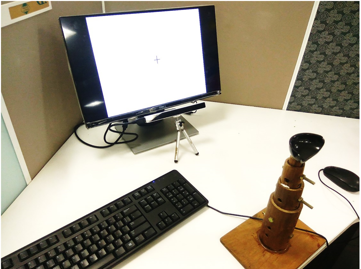
Fig 9. Experimental setup with the eye tracker at the bottom of the display and a chin rest.
