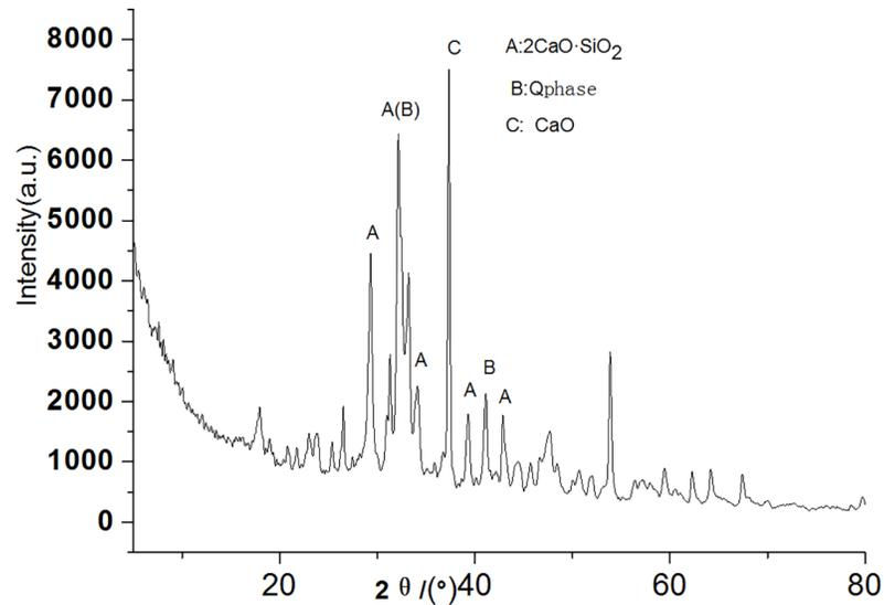
Fig 9. XRD spectra for the major mineral components of the clinker sample M7.
