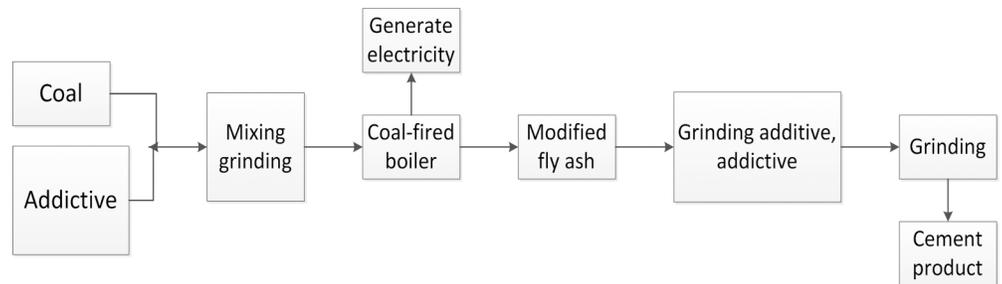
**Fig 1. Diagram of the coproduction process of cement clinker in a power plant pulverized coal boiler.**
