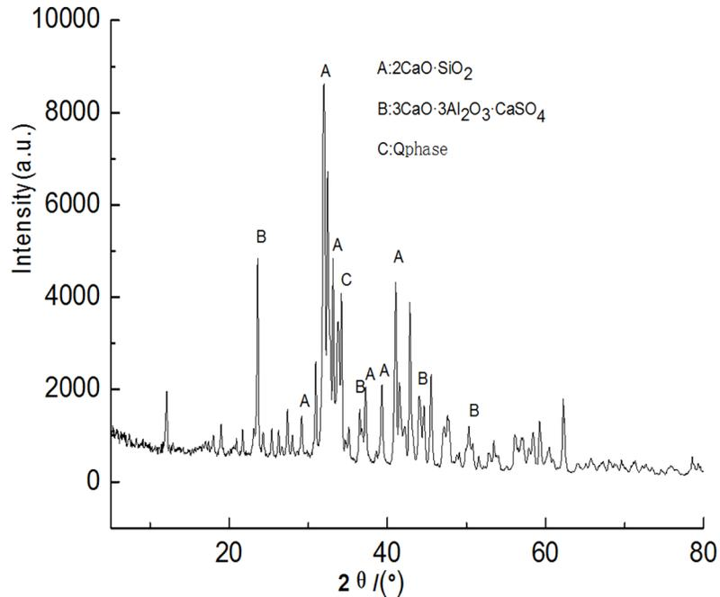
Fig 7. XRD spectra for the major mineral components of the clinker sample M5.
