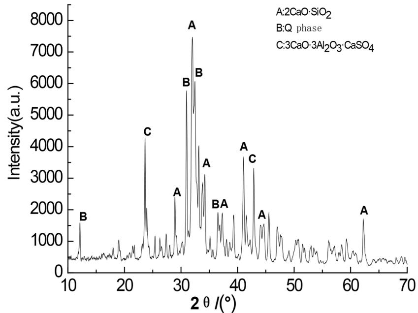
Fig 3. XRD spectra for the major mineral components of the clinker sample M1.
