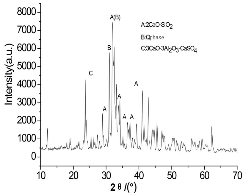
Fig 4. XRD spectra for the major components of the clinker sample M2.
