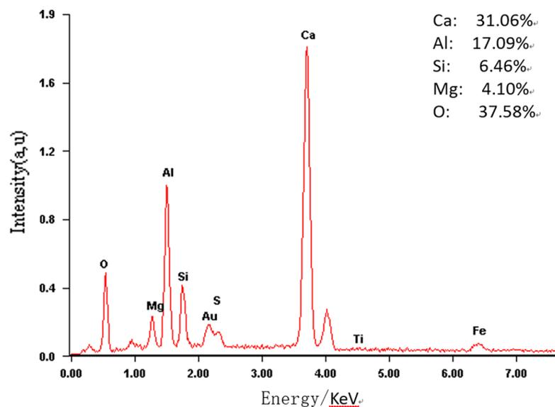
Fig 12. The EDS micrograph of the Q phase in mixed pulverized coal M2.
