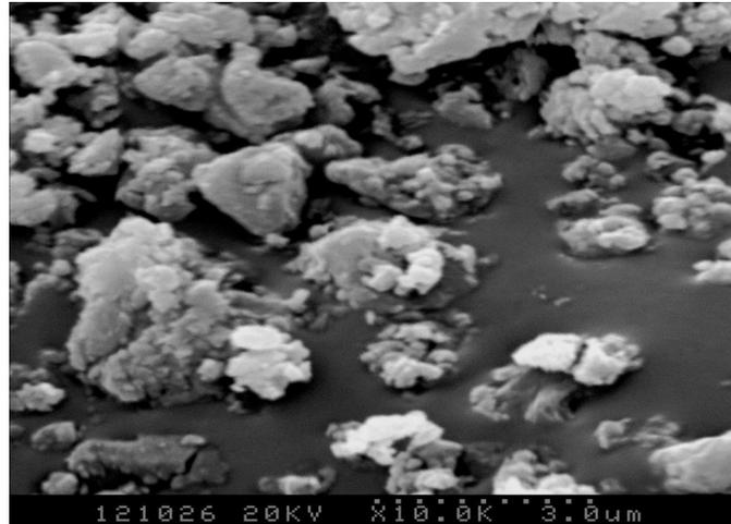
Fig 11. The SEM micrograph of globular mixed pulverized coal M3.
