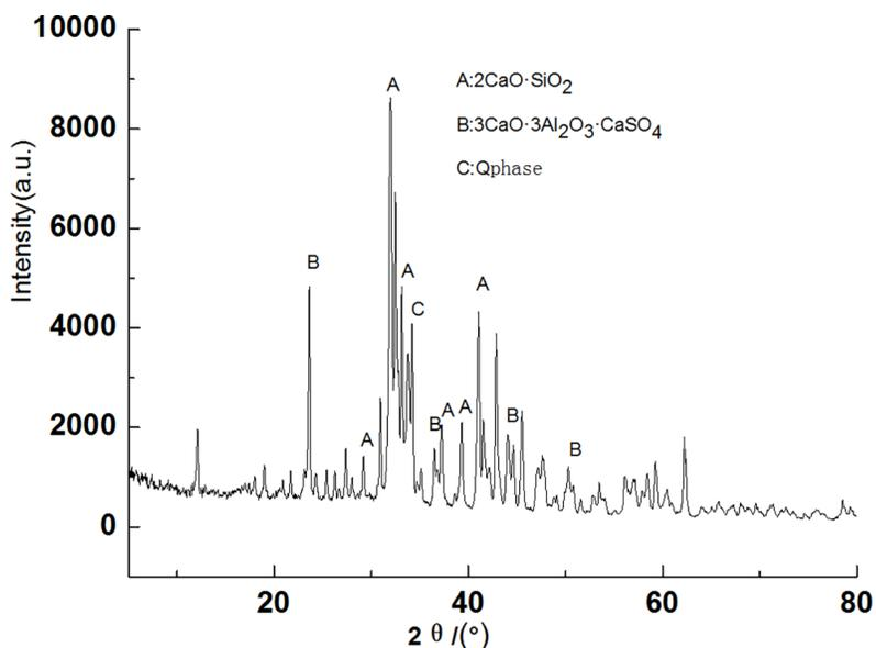
Fig 6. XRD spectra for the major mineral components of the clinker sample M4.
