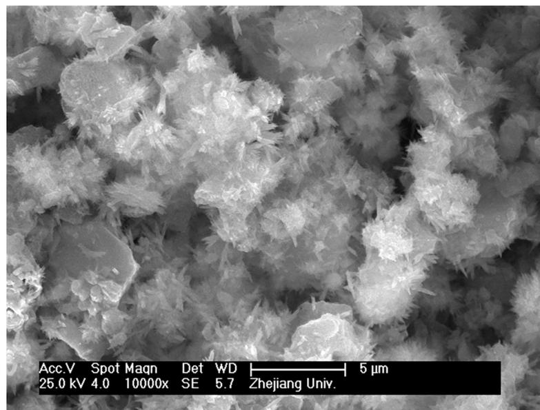
Fig 10. The SEM micrograph of globular mixed pulverized coal M2.
