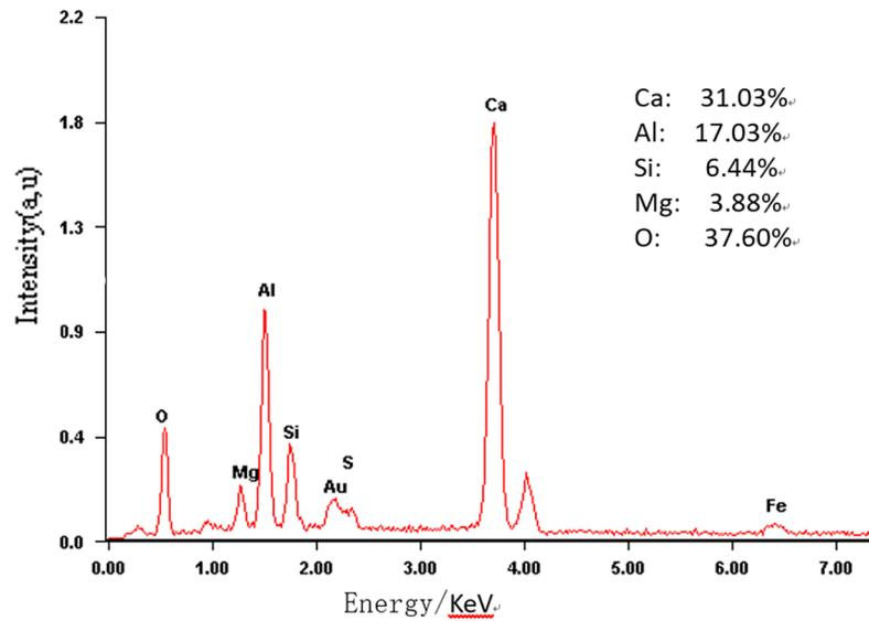
Fig 13. The EDS micrograph of the Q phase in mixed pulverized coal M3.
