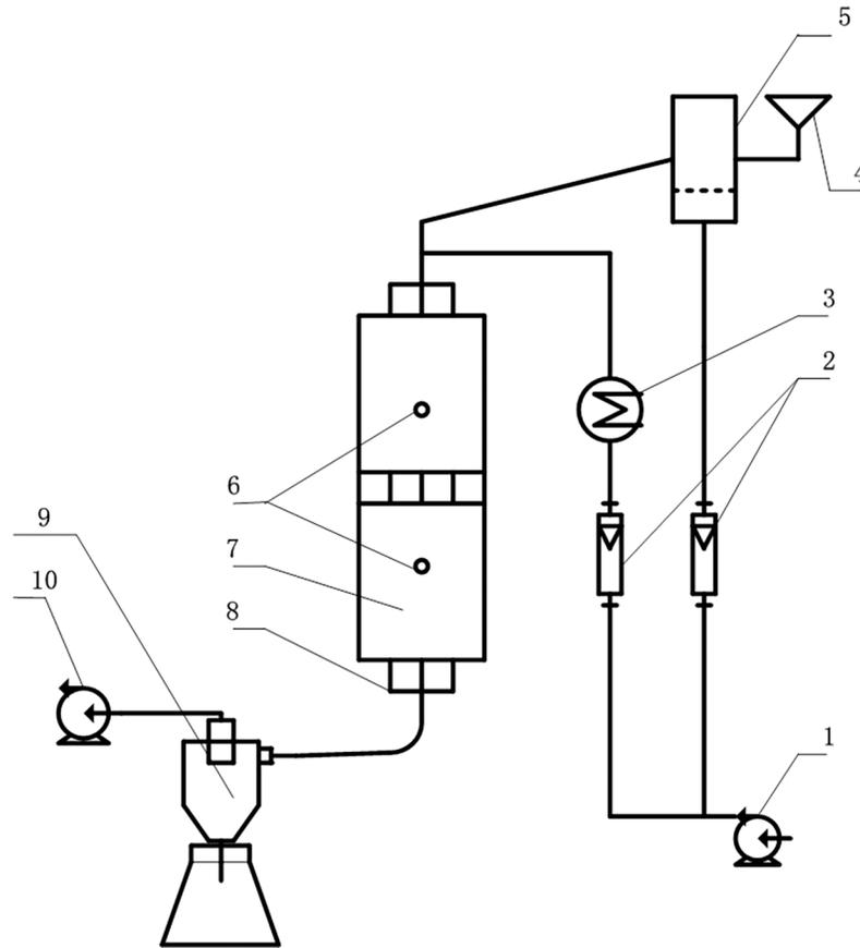
**Fig 2. Diagram of two-stage multiphase reaction test bed.** 1: Air compressor 2: Rotor flow meter 3: Air preheater 4: Gunk 5: Fluidized bed feeder 6: Thermocouple 7: Furnace body 8: Water-cooled jacket 9: Cyclone dust collector 10: Induced draft fan.
