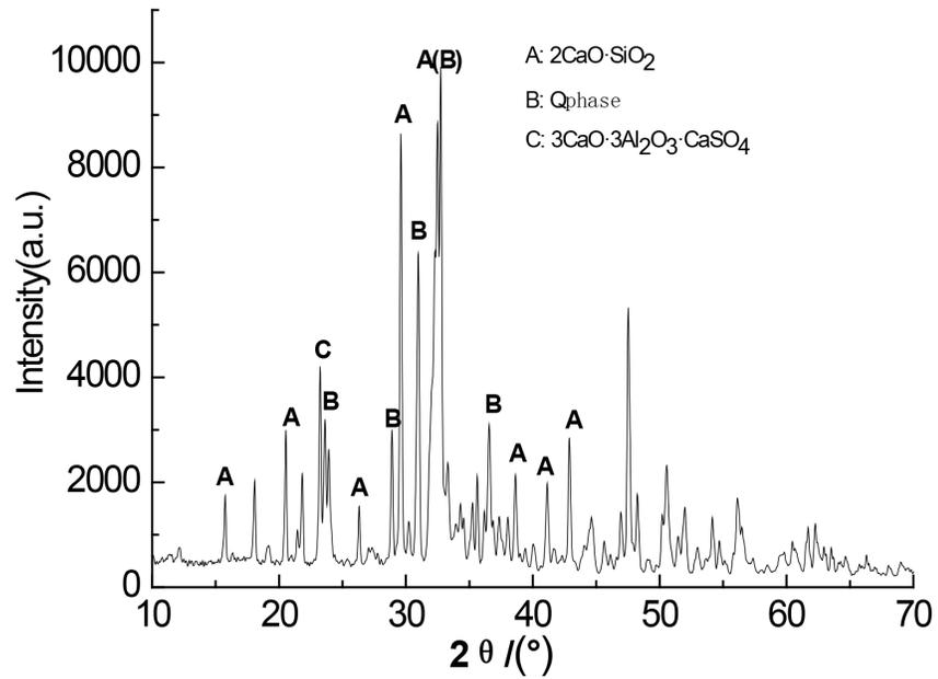
Fig 5. XRD spectra for the major mineral components of the clinker sample M3.
