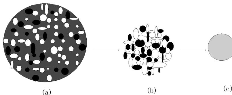
Fig 14. The process diagram for the formation of cement clinker particles from mixed coal powder globular polymerized particles. (a)The moment of the ultra-fast temperature rise of the mixed coal powder globular polymerized particle. (b)Combustible burning and decomposition and aggregation of inorganic mineral. (c)The formation reaction of clinker minerals.
