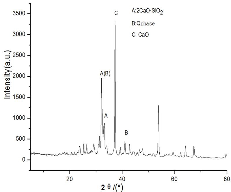
Fig 8. XRD spectra for the major mineral components of the clinker sample M6.
