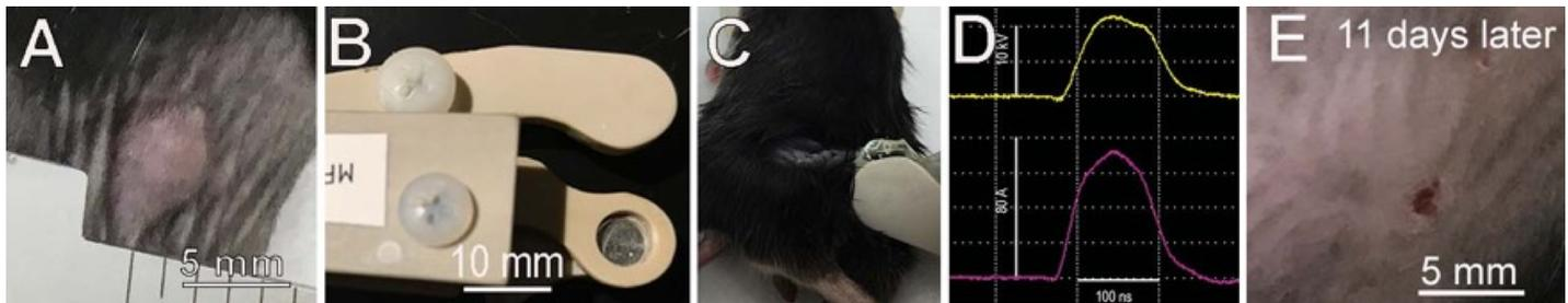
**Fig 1. NPS application.** (A) Photo of a typical shaved C3.43 tumor prior to treatment. (B) Pinch electrode used to treat these tumors. (C) Pinch electrode sandwiching a tumor as NPS is applied. (D) Oscilloscope trace of voltage (top) and current (bottom) applied to the tumor in each pulse. (E) Photo of the treated tumor in “A” 11 days later.
