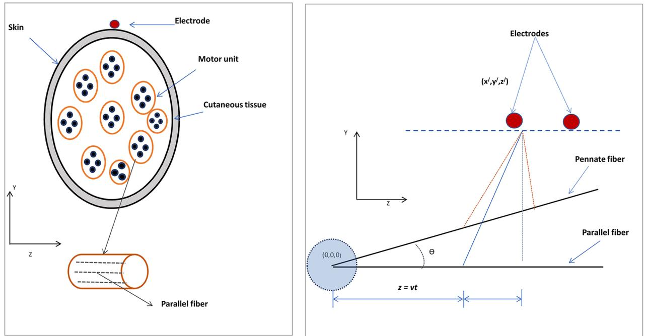
**Fig 1. Representation of EMG model: a) position of motor units of muscle with respect to electrode located at skin, b) position of parallel fibre and pennate fibre with respect to electrode.**
