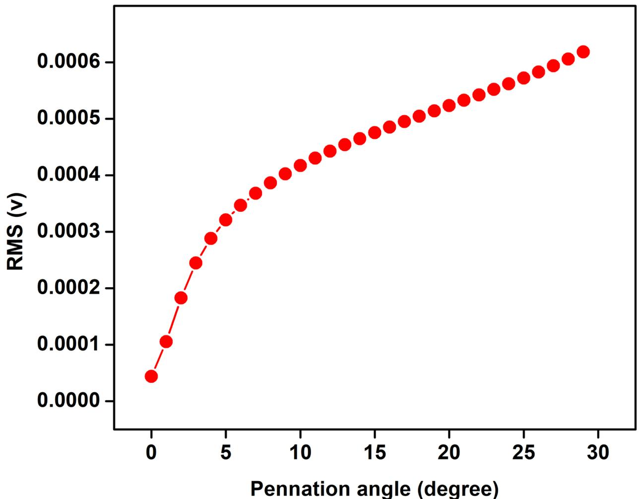
**Fig 4. Change in sEMG amplitude with variation in pennation angle.**
