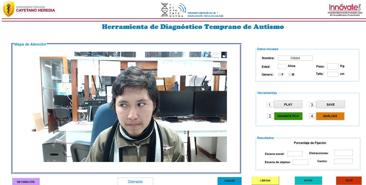
Fig 6. Graphical user interface of the eye-tracking tool, demonstrating the patient data input, the main controls for the video display and video capture, and visual preference data output. Demonstration of the frame-by-frame analysis for visual preference by displaying pupil position for both eyes, allowing for investigator corroboration.
