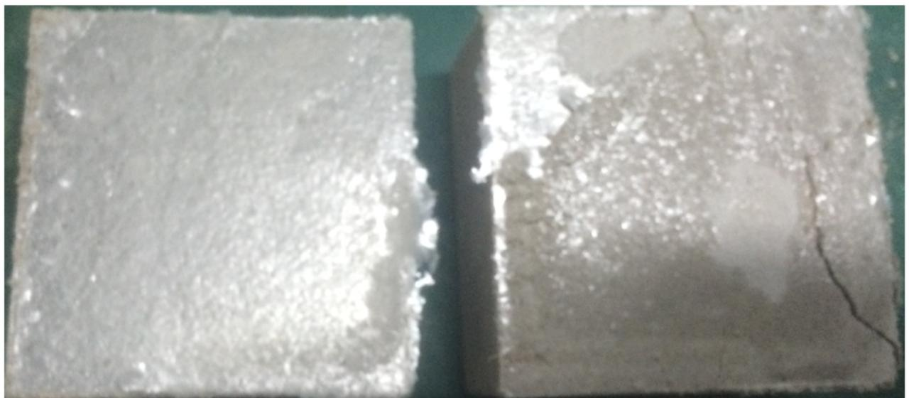
**Fig 3. Failure mode of a flat joint with direct shear.**
