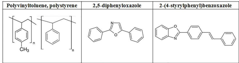
**Fig 2. Components of the J-PET plastic scintillators.**
