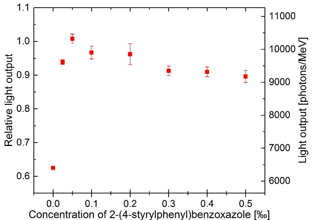
**Fig 8. Relative and absolute light output of the J-PET plastic scintillators.**
