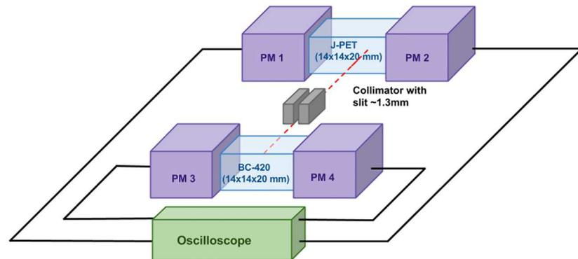
**Fig 4. Scheme of the experimental setup for the J-PET scintillators tests.** PM denotes photomultiplier. As oscilloscope a Serial Data Analyser (Lecroy SDA6000A) was used. It allowed to collect waveforms of four photomultipliers' signals simultaneously with the sampling interval of 100 ps.
