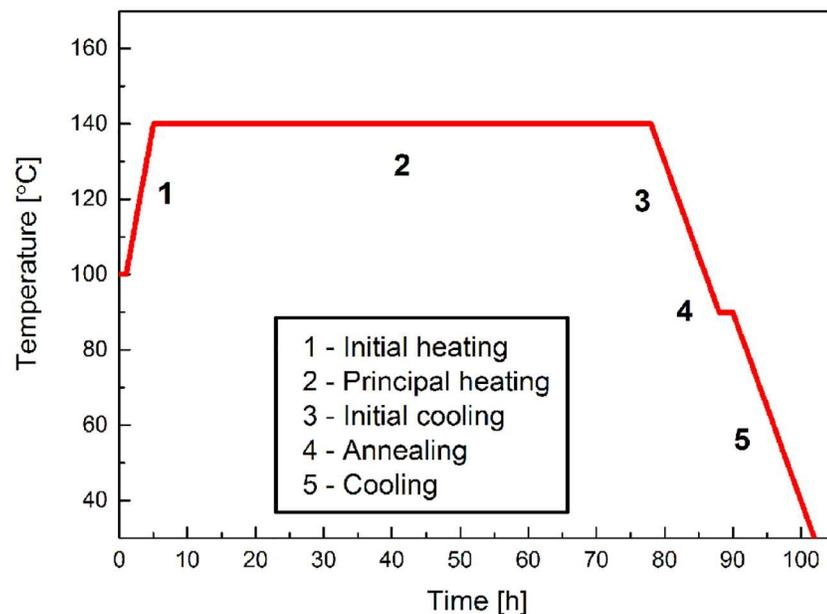
**Fig 3. Thermal schedule for scintillator polymerization.**
