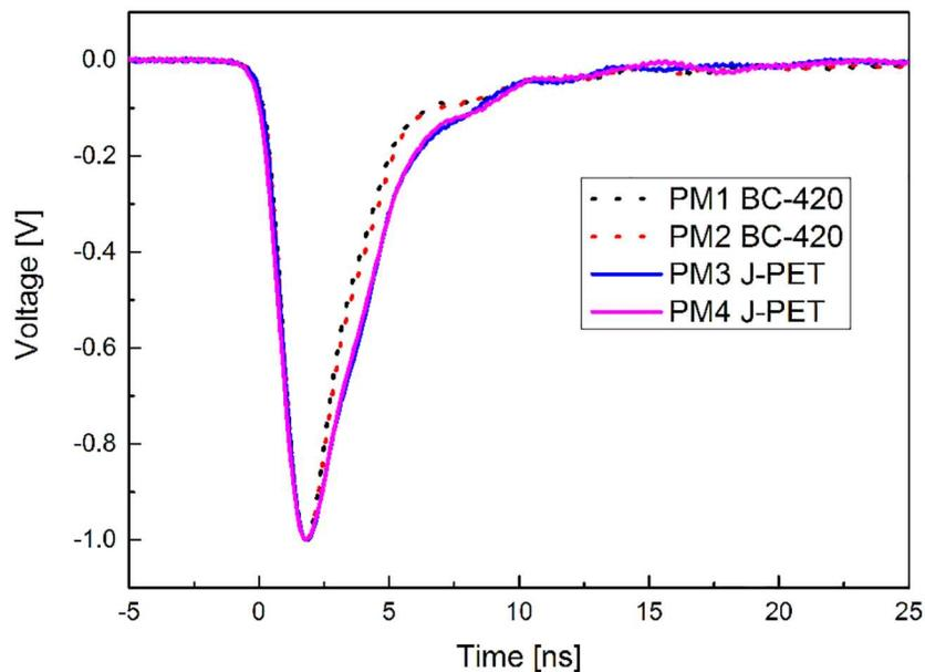
**Fig 9. Average signals measured with detectors consisting of the BC-420 or the J-PET scintillators and Hamamatsu R9800 photomultiplier.** The shown shapes result from averaging of  $10^5$  signals using method described in references [17]. Signals were normalized to the amplitude equal to 1V.
