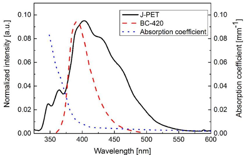
**Fig 6. Emission spectra of BC-420, J-PET scintillator and scintillators' absorption coefficient  $\mu_{eff}$  [37, 38].** The emission spectra are normalized in amplitude.
