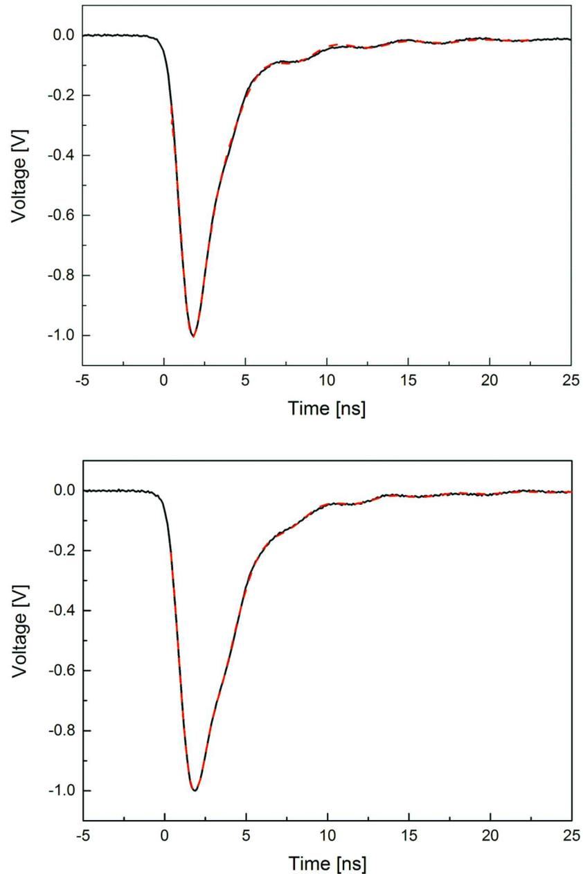
**Fig 10. Averaged signals from photomultiplier connected to BC-420 scintillator (top) and to J-PET scintillator (bottom).** Red dashed line indicates result of fitting a function given by the sum of Formulas (2) and (3). Signals were normalized to the amplitude equal to 1V.
