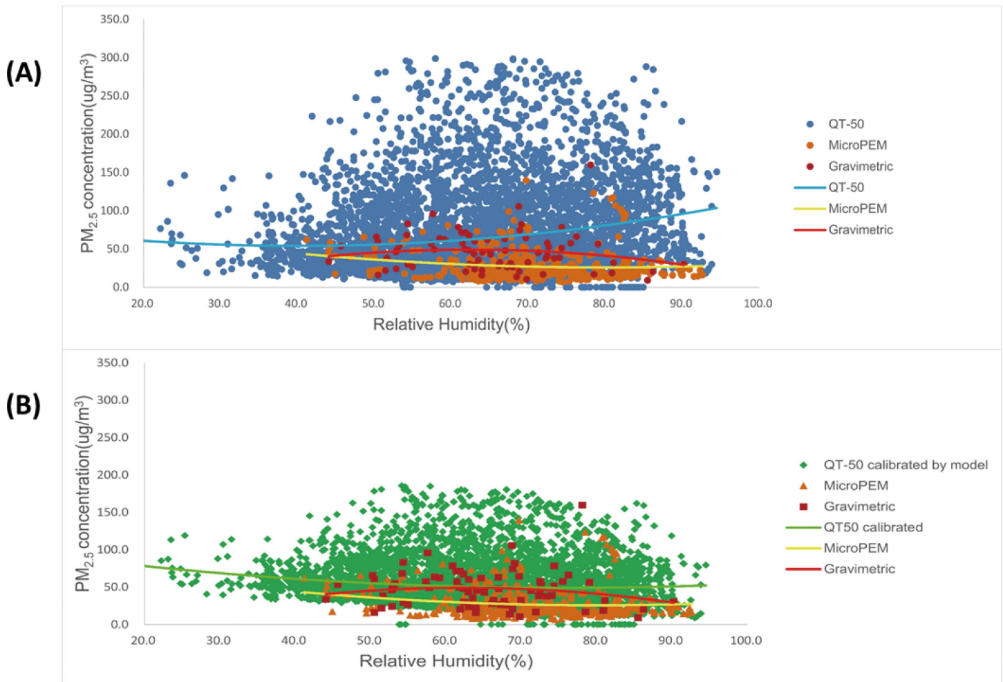
Fig 3. The distribution of PM 2.5 concentration by QT-50, MicroPEM and gravimetric method at different RH before QT-50 calibration (A) and after calibration (B). In both Fig 3(A) and Fig 3(B), each point refers to a PM 2.5 concentration data and the lines refer to the PM 2.5 trend by RH. The points by QT-50 and MicroPEM were the original 10-min data of PM 2.5 . The points indicated as “Gravimetric” were the integrated average in each sample by SKC pumps. Y axis refers to the PM 2.5 concentration level (μg/m 3 ) and X axis refers to RH.
