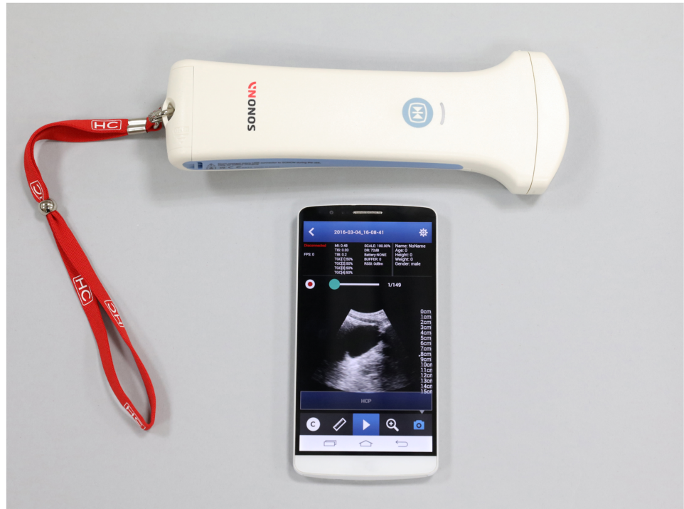
Fig 1. Photograph of the pocket-sized ultrasound device. Images were displayed on a smartphone via a device-generated wireless (free Wi-Fi) connection. Under a Creative Commons (CC) license permission to publish this picture was obtained from HEALCERION, Seoul, Korea (S2 File).
