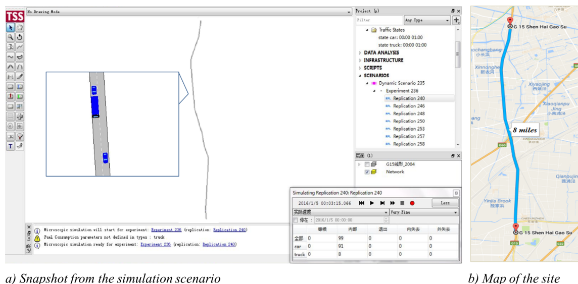
Fig 6. Aimsun interface of the simulated section.
