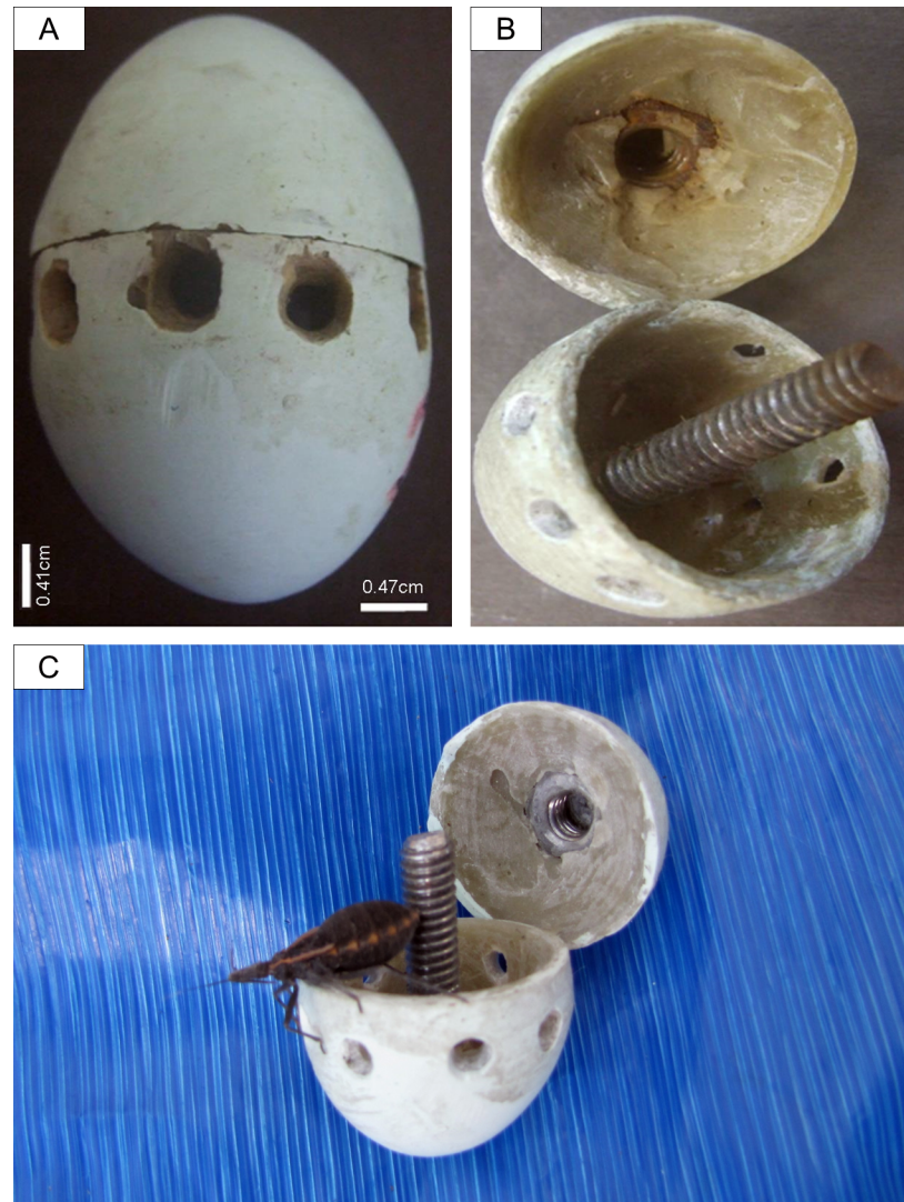
Fig 1. Fake eggs and hematophagous insects used for blood collection of incubating cattle egret adults. Photograph showing: (A) Side view of fiberglass egg mimicking cattle egret egg (approximate dimensions: 45 mm length, 33 mm width) with holes through which the insect projects its proboscis; (B) Interior view of two halves of egg, which are attached with nut and bolt; (C) Fifth instar Panstrongylus megistus larva being removed from a fake-egg after having fed on an incubating cattle egret. Note the insect's engorged abdomen.
