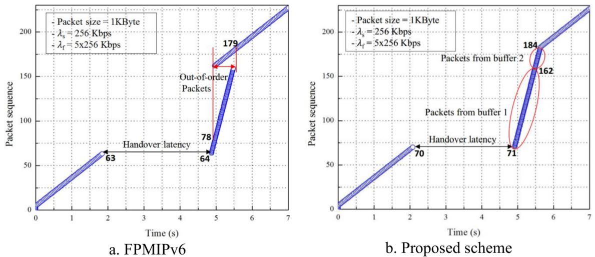
Fig 11. Packet flow with  $\lambda_s = 256$  Kbps,  $\lambda_r = 5\lambda_s$ . (a) FPMIPv6, (b) Proposed scheme.
