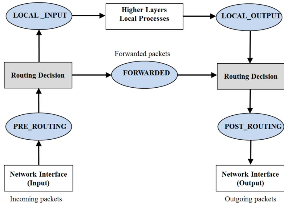
**Fig 5. Netfilter hooks and packet flow.**
