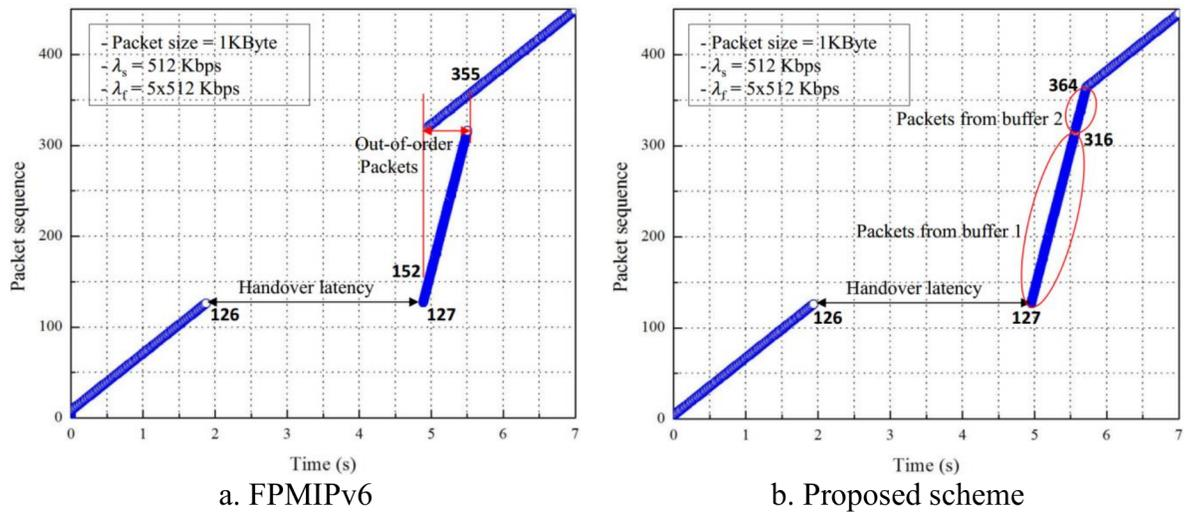
**Fig 12. Packet flow with  $\lambda_s = 512$  Kbps,  $\lambda_f = 5\lambda_s$ .** (a) FPMIPv6, (b) Proposed scheme.
