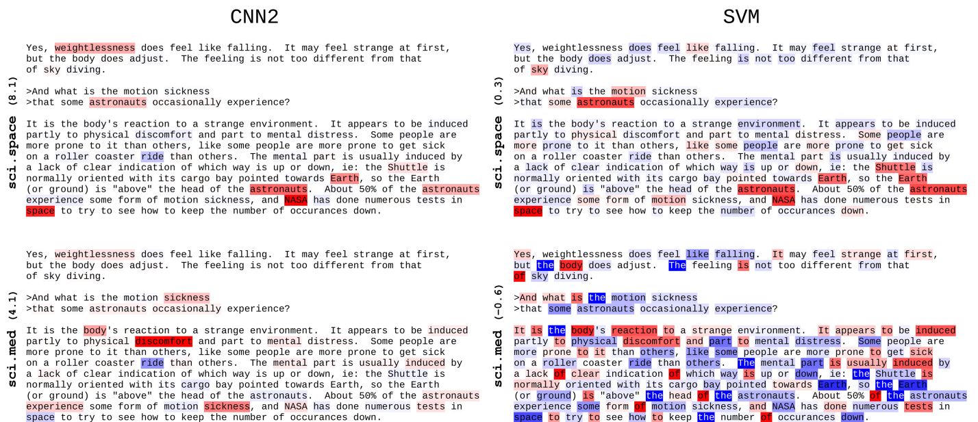
Fig 2. LRP heatmaps of the document sci.space 61393 for the CNN2 and SVM model. Positive relevance is mapped to red, negative to blue. The color opacity is normalized to the maximum absolute relevance per document. The LRP target class and corresponding classification prediction score is indicated on the left.
