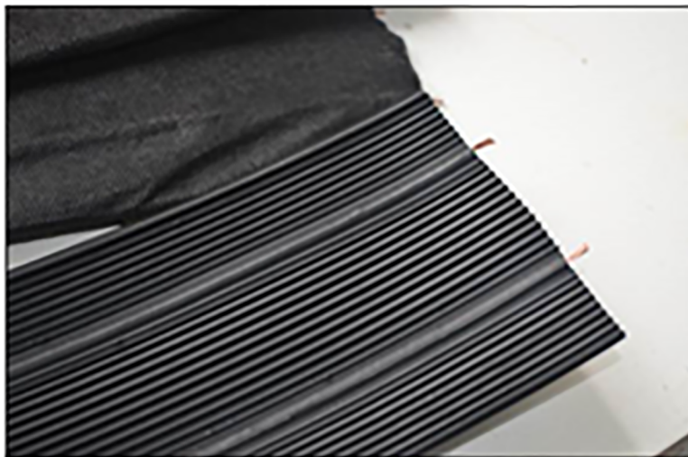
Fig 2. Real product of the EKG electrode. The functions of EKG materials included drainage, electric conduction and corrosion resistance. This new material can relatively shorten the consolidation time when compared with the conventional test and can also avoid the electrolytic reaction of metal electrodes during the test. Thus, the EKG can make the coupling between the electric seepage field and the hydraulic seepage field more effectively.
