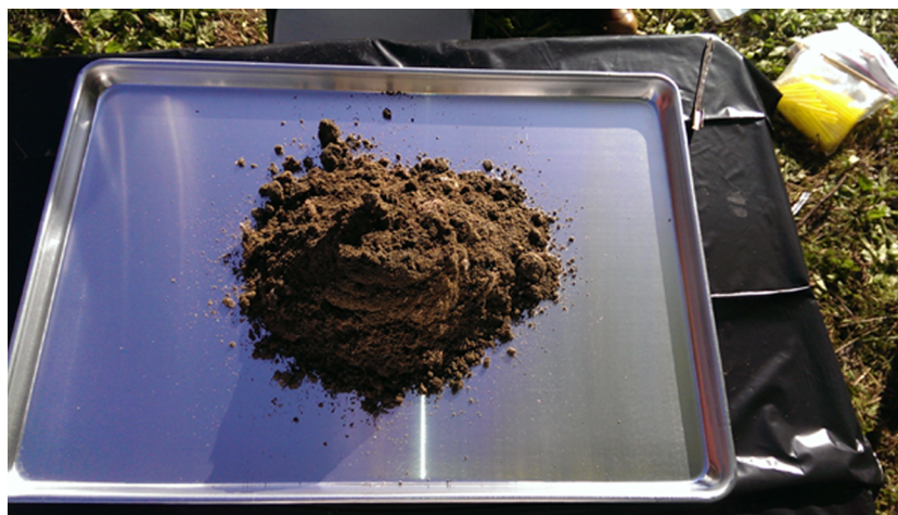
Fig 4. ISM soil sample spread out on aluminum baking tray.
