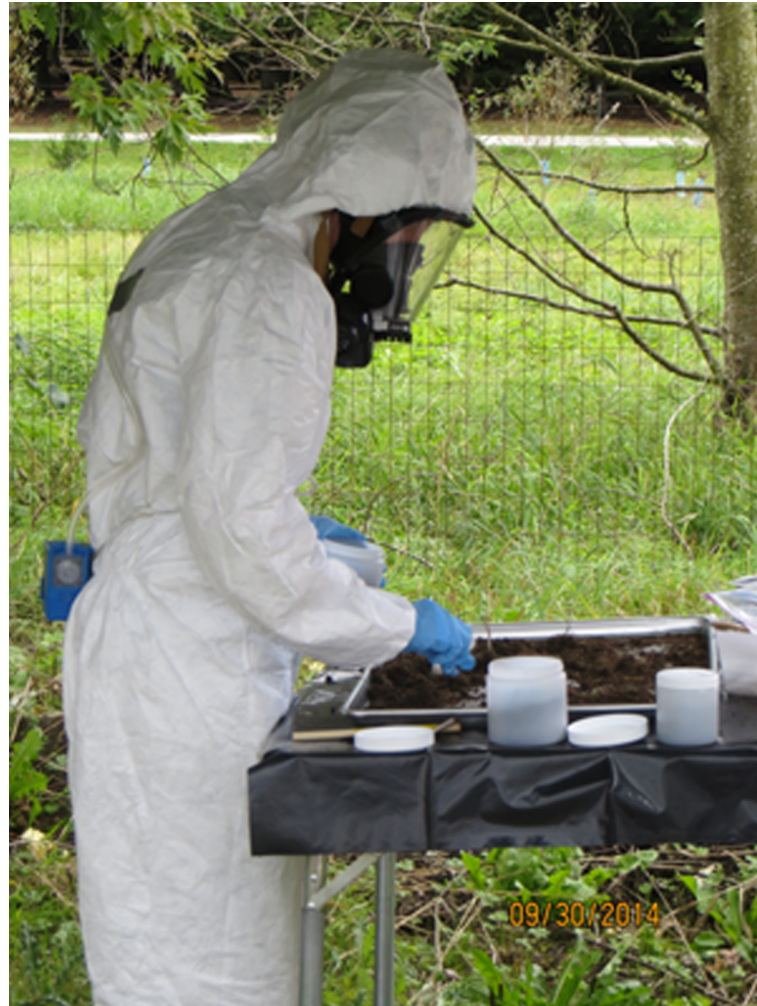
Fig 7. Breathing zone sample being collected during ISM subsampling.
