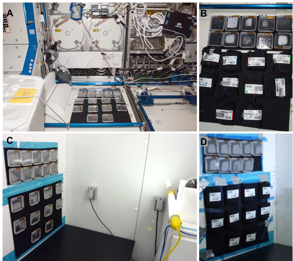
Fig 1. Experiment configuration and growth habitats. (A) The flight plates attached to the wall of the Destiny module of the International Space Station. (B) After germination was initiated by exposure to light, the dark-grown plates were re-wrapped in Duvetyne Black-Out cloth. (C) The ground control plates attached to the wall of the ISS Environment Simulations (ISSES) chamber at Kennedy Space Center in a vertical orientation for growth. (D) The dark-grown plates in the ISSES chamber after re-wrapping.
