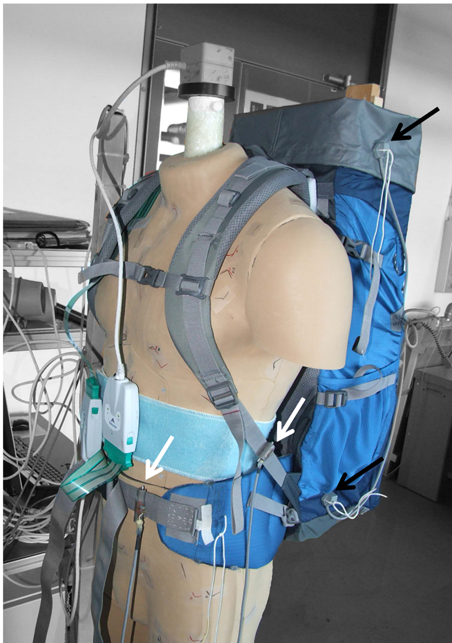
Fig 3. Dummy with load carriage system. The strap force sensors are mounted in the shoulder strap and the hip belt (white arrows). The Polhemus LIBERTY source is mounted on top of the dummy and its sensors are at the top and the bottom of the load carriage system (black arrows).
