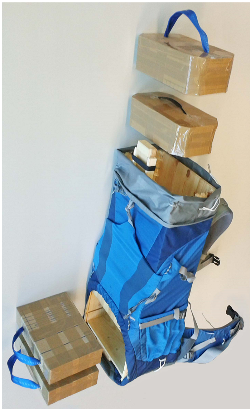
Fig 2. Load carriage system. Cardboard boxes filled with sand could be inserted through an opening in the backpack and the wooden box at the bottom and the top to enable efficient change of the payload, while keeping the center of mass in the same position.
