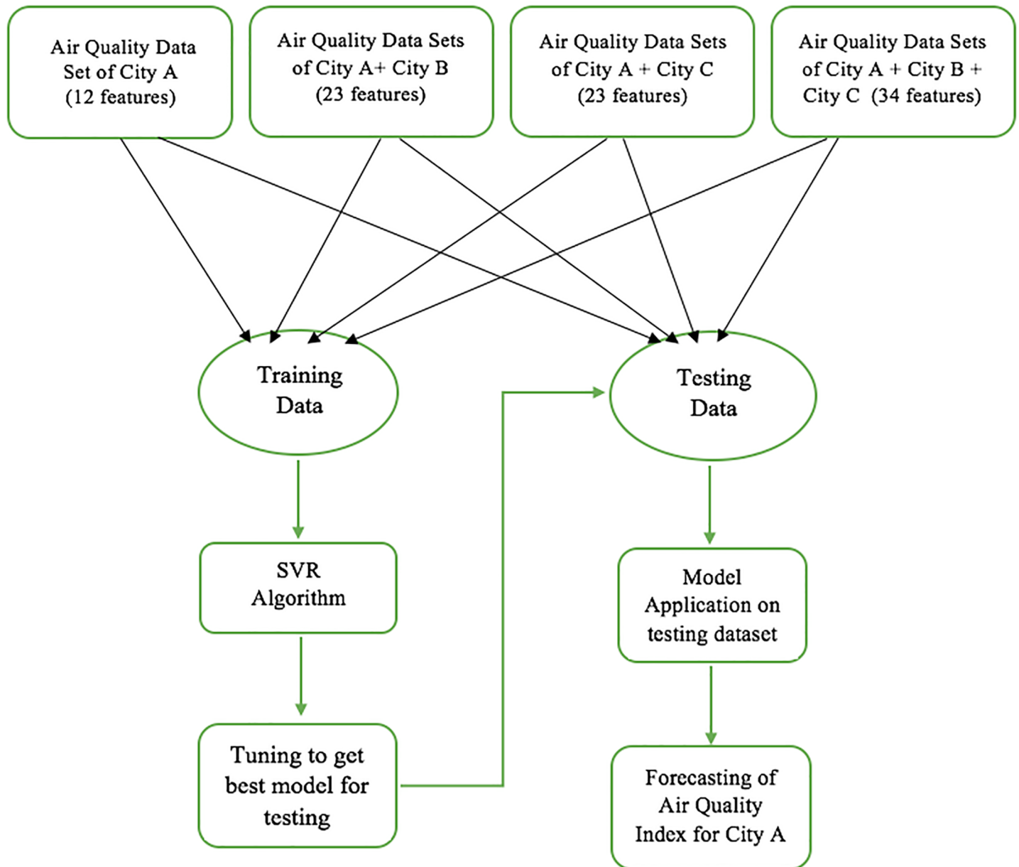
Fig 3. Multi-dimensional codimensional collaborative SVR Model for forecasting AQI values of City A using air quality data sets of city A + city B, city A + city C, city A + city B + city C.
