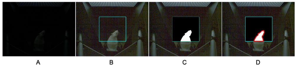
**Fig 8. Illustration of image preprocessing steps.** A: Original image (Resolution: 640 × 480). B: Gamma correction ( $A = 1.0, \gamma = 3.3$ ; The highlighted rectangle denotes the manually selected ROI). C: Binarization (threshold detected automatically with Otsu's method). D: Contour extraction. The red boundary is the extracted contour.
