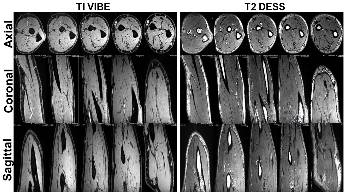
Fig 3. 7T T1 VIBE and T2 DESS images of the forearm demonstrating homogeneous excitation in axial [elbow to wrist], coronal and sagittal planes. The B1+ field coefficient of variation was calculated to be 21% in the forearm [encapsulated within the coil volume].
