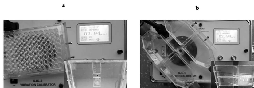
Fig 2. (a)Vibration sensor with fixator for culture plates, and(b) vibration sensor with fixator for culture flasks.
