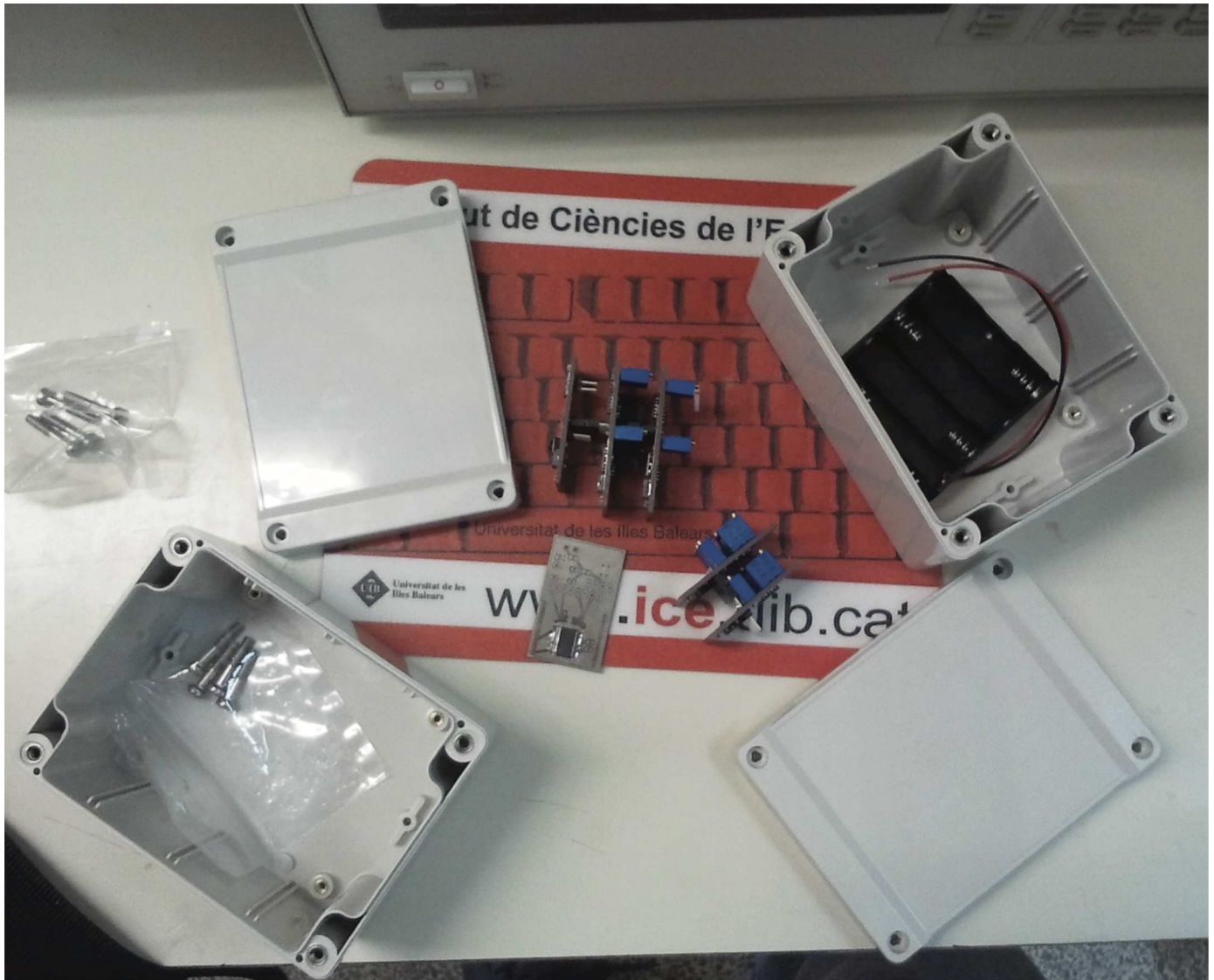
Fig 6. Electronic device for wireless transmission: Enclosure box and batteries.
