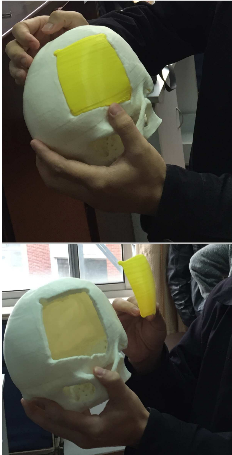
Fig 14. The photo shows the inspection of a 3D printed implant (yellow) and the corresponding 3D printed patient skull (white), which has a large defect on the left side.
