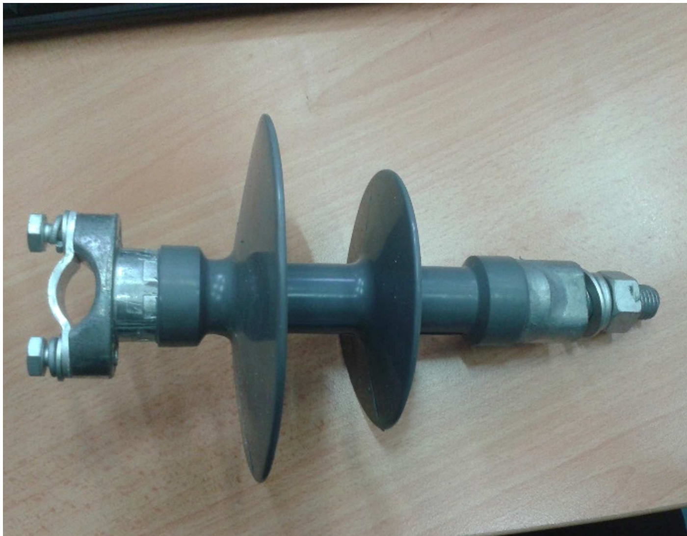
Fig 5. Typical 10kV polymer insulator.
