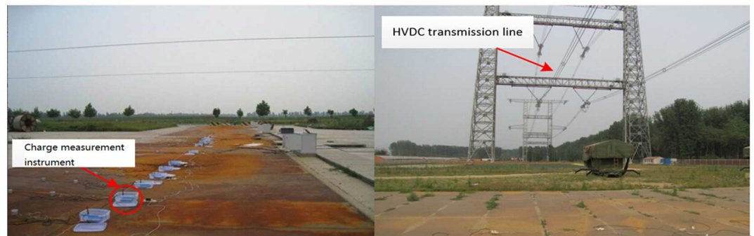
Fig 11. Picture of measurement system in HVDC test base.
