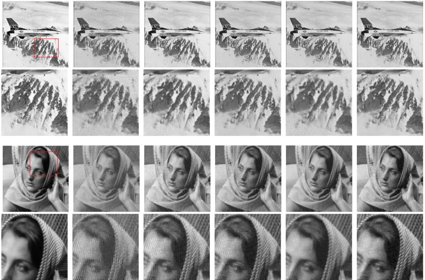
Fig 6. Reconstructed images by pseudo-radial sampling. From top to bottom for each column: Plane image, close-up of the red rectangle of Plane image, Barbara image, close-up of the red rectangle of Barbara image. From left to right for each row: the original image, the TV method, the NLR-CS-baseline method, the NLR-CS method, the BM3D-CS method, the proposed method.
