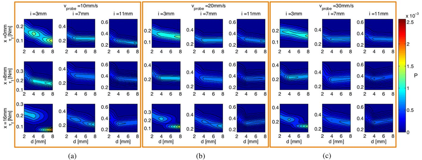
**Fig 6. Examples of memory primitives computed as probability functions of the de-noised torque profiles from 25 trials given different interaction conditions shown in Table 3.** The sample of memory primitives shown here consist of those when the PSV,  $v_{probe} = 10, 20,$  and  $30,$  in subfigures (a), (b), and (c), for the indentation level,  $i,$  of  $3, 7,$  and  $11$  mm, and the stiffness of the joint denoted by  $r_a,$  of  $0, 8,$  and  $16$  mm.
