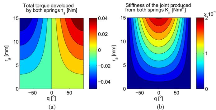
**Fig 3. Simulated joint torque and stiffness.** Torque (a) and the stiffness (b) produced at the pivot joint due to the changes in the displacement of the anchor ring,  $r_a$ , and the angular displacement of the joint,  $q$ .
