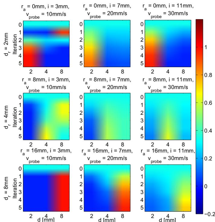
**Fig 7. Examples of posterior distribution of nodule's depth estimation across iterations.** Each plot depicts the distribution of depth estimation from the initially defined flat distribution at  $t = 0$  to  $t = 5$  given different combinations of probe's stiffness, indentation, and PSV. The real depths of nodule,  $d_r$ , assessed here were those known values associated with the memory primitives explained earlier.
