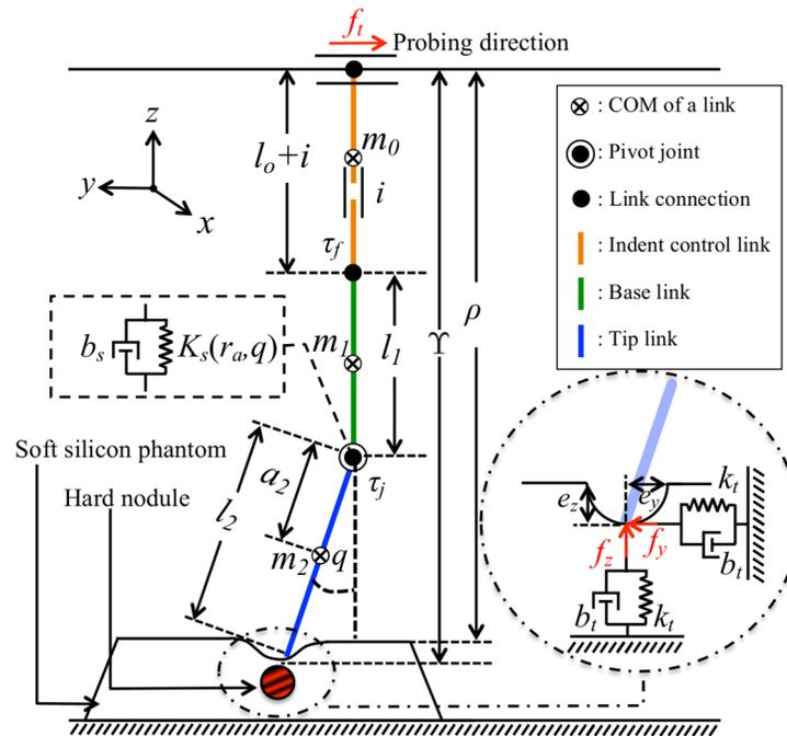
**Fig 4. Schematic view of the probe interacting with simulated softsilicon phantom.** The probe consists of two rigid manipulator links with a variable stiffness joint. In the experiment,  $\tau_f$  is measured at the end of base link of the probe using ATI Nano17. The nodule embedded inside the phantom is shown in red-black spherical ball. The physical properties of phantom is described using spring-damper system. The variables used in the system is described in [Table 1](#).
