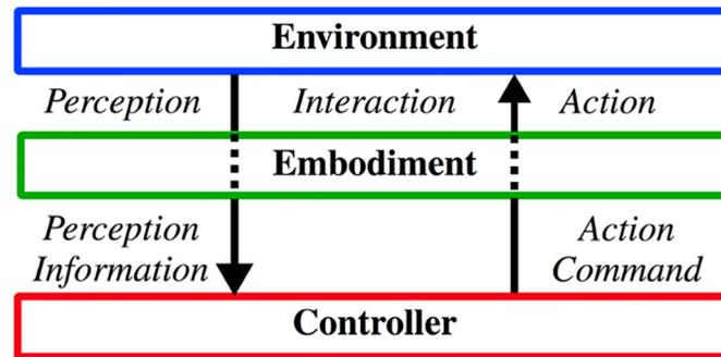
**Fig 1. Embodiment mediates both perception and action during the interaction between an agent and the environment.** The system interacts with the environment through its embodiment. The internal impedance required for accurate perception through its embodied sensor can differ from that required to take appropriate action. Likewise an action taken with appropriate impedance could affect the quality of perception of the environment.
