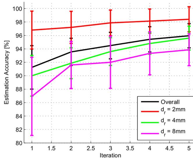
**Fig 8. The nodule’s depth estimation accuracy under fixed-5-iteration Bayesian inferencing algorithm.** The resulting overall nodule’s depth estimation accuracy is shown in black line. The estimation accuracy for each actual depth,  $d_r = 2, 4,$  and  $8\text{ mm}$  are shown in red, green and magenta lines respectively.
