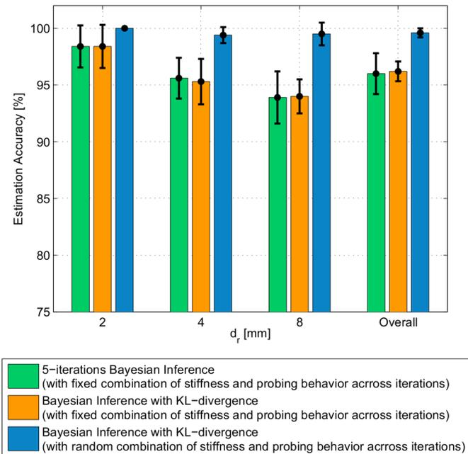
**Fig 9. Overall nodule’s depth estimation accuracy when using different approaches.** 1) 5-iteration Bayesian inference without KL-divergence (shown in green), 2) the Bayesian Inference together with the KL-Transfer Entropy with fixed probe’s stiffness, indentation level, and PSV (shown in orange), and 3) the Bayesian Inference together with the KL-Transfer Entropy with random probe’s stiffness, indentation level, and PSV (shown in blue).
