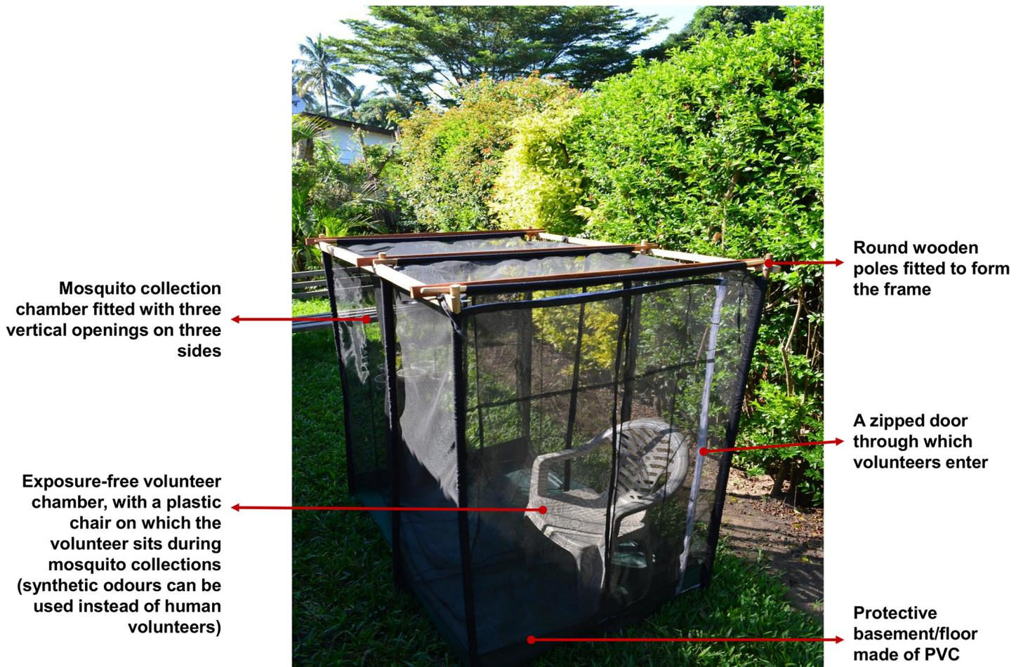
**Fig 3. The M-Trap.** Pictures of the odour-baited trap, the M-trap, used for comparative assessment of mosquito densities. Vertical envelope-shaped mosquito entry points are labelled. In our study, no human volunteer occupied the trap, and instead we relied on synthetic mosquito attractants complemented with carbon-dioxide gas.
