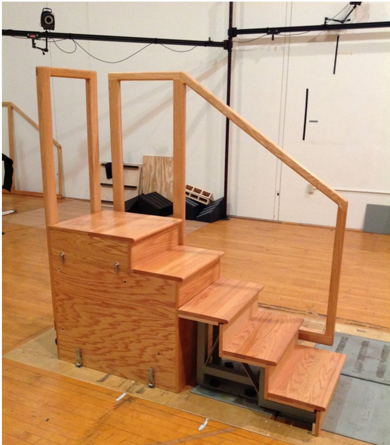
Fig 1. The 5-step (3 instrumented and 2 for turning around) staircase securely bolted to two force platforms for experimental data collection of ground reaction forces during stair negotiation.
