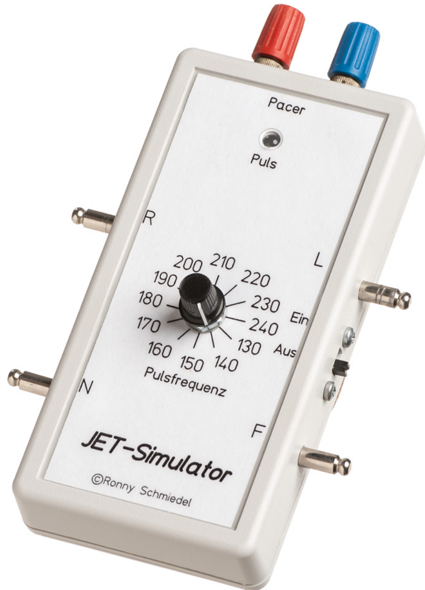
Fig 2. The custom-made JET simulator. JET rates are selected via a rotary switch in the middle of one face. Signals for an ECG monitor are provided at the lateral output sites. Output plugs at the top supply the input signal for the pacemaker. An on/off switch is located at the right side of the device. R: right, L: left, F: foot, N: neutral.
