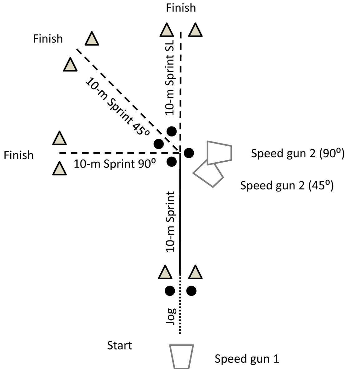
**Fig 1. Experimental set up with the new timing methodology combining two speed guns synchronized.** See [methods](#) for details.
