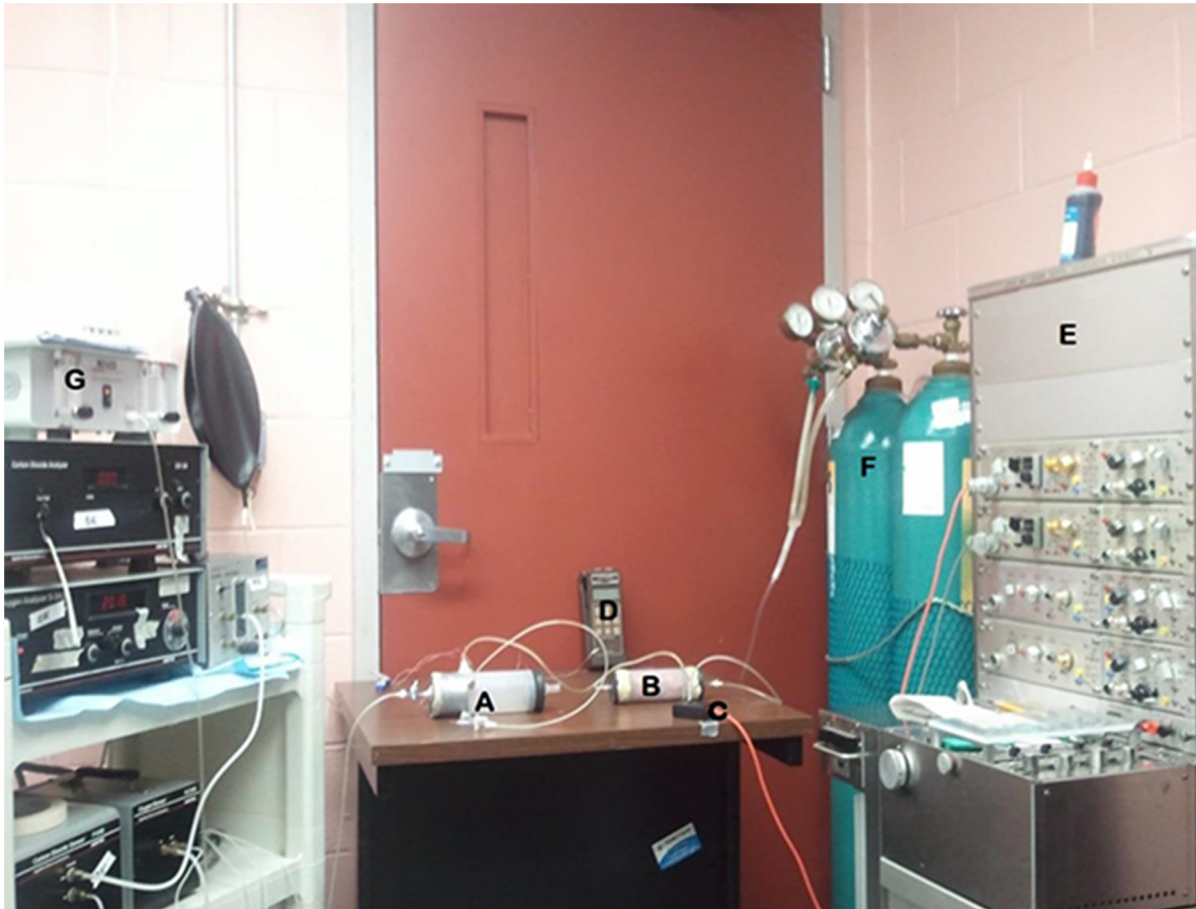
Fig 1. Modified Barometric Plethysmography. Photograph of plethysmography set up for ventilatory function analysis. (A) Animal chamber; (B) Reference chamber; (C) Transducer; (D) Thermometer; (E) Polygraph machine; (F) Gas mixture; (G) Flow meter.
