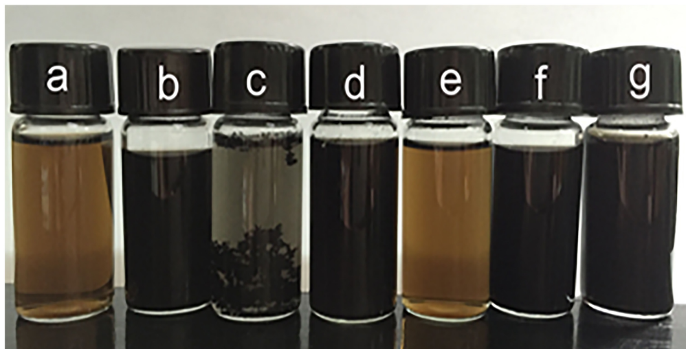
Fig 1. Photograph of the samples ( 0.1 \text{ mg}\cdot\text{mL}^{-1} , GO (a) and RGOs (L-AA RGO-1 (b), L-AA RGO-2 (c), D-GLC RGO-1 (d), D-GLC RGO-2 (e), N RGO (f), and TP RGO (g)).
