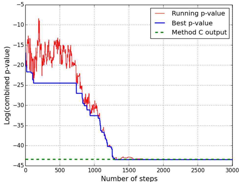
Fig 9. Example of simulated annealing search. A single run of SA stochastic search for the global minimum p-value, applied to the pH = 5 vs pH = 7 comparison microarray dataset. Sharp fluctuations in the red curve arise from the possibility of non-optimal updates, the propensity for which depends on the (gradually decreasing) annealing temperature.
