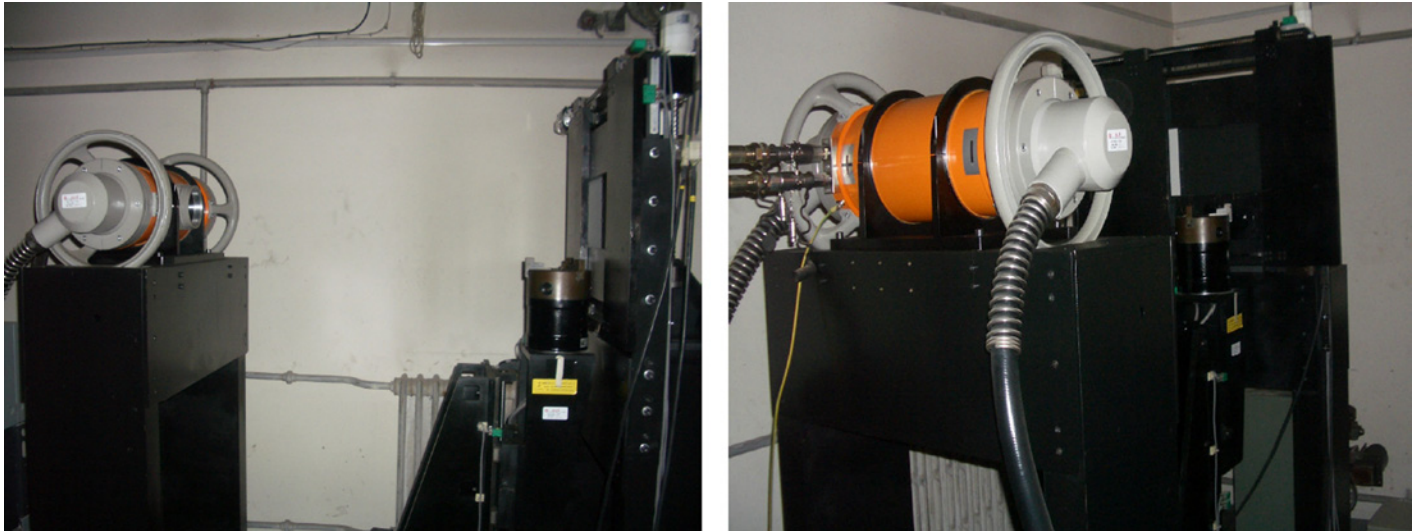
Fig 4. The experiment CT system. This system is composed by X-ray (GE ISOVOLT 450KV) and detector (VARIAN PaxScan2520).
