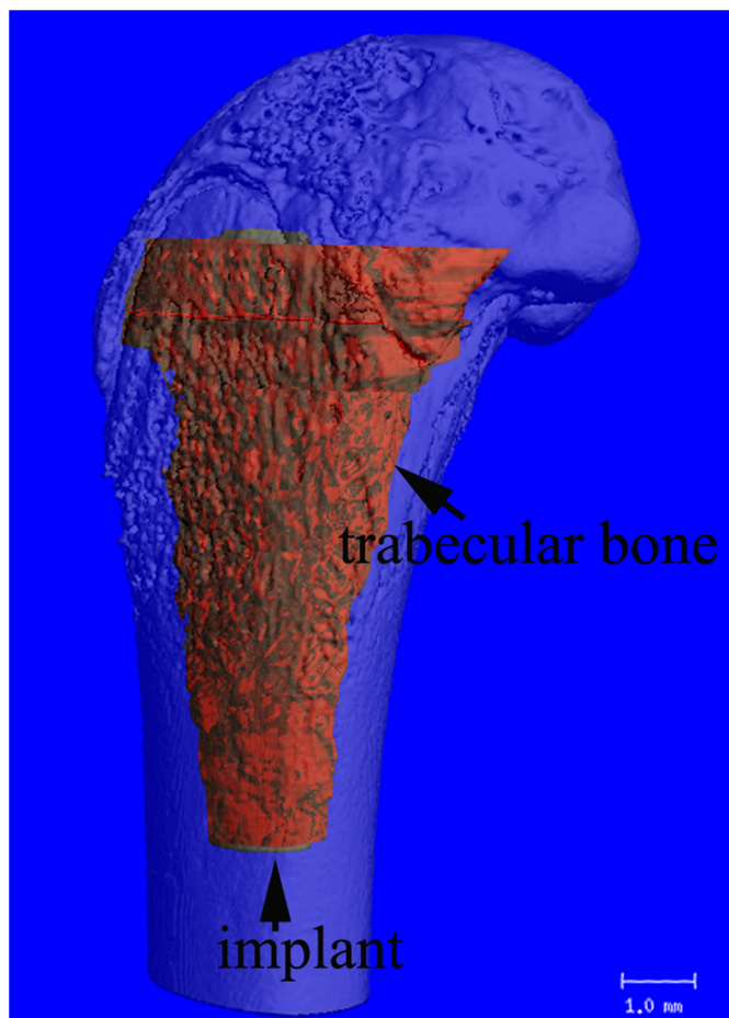
Fig 2. A 3D image illustrating the precise region of interest (trabecular bone between the implant and cortex, red region) evaluated by micro-CT.
