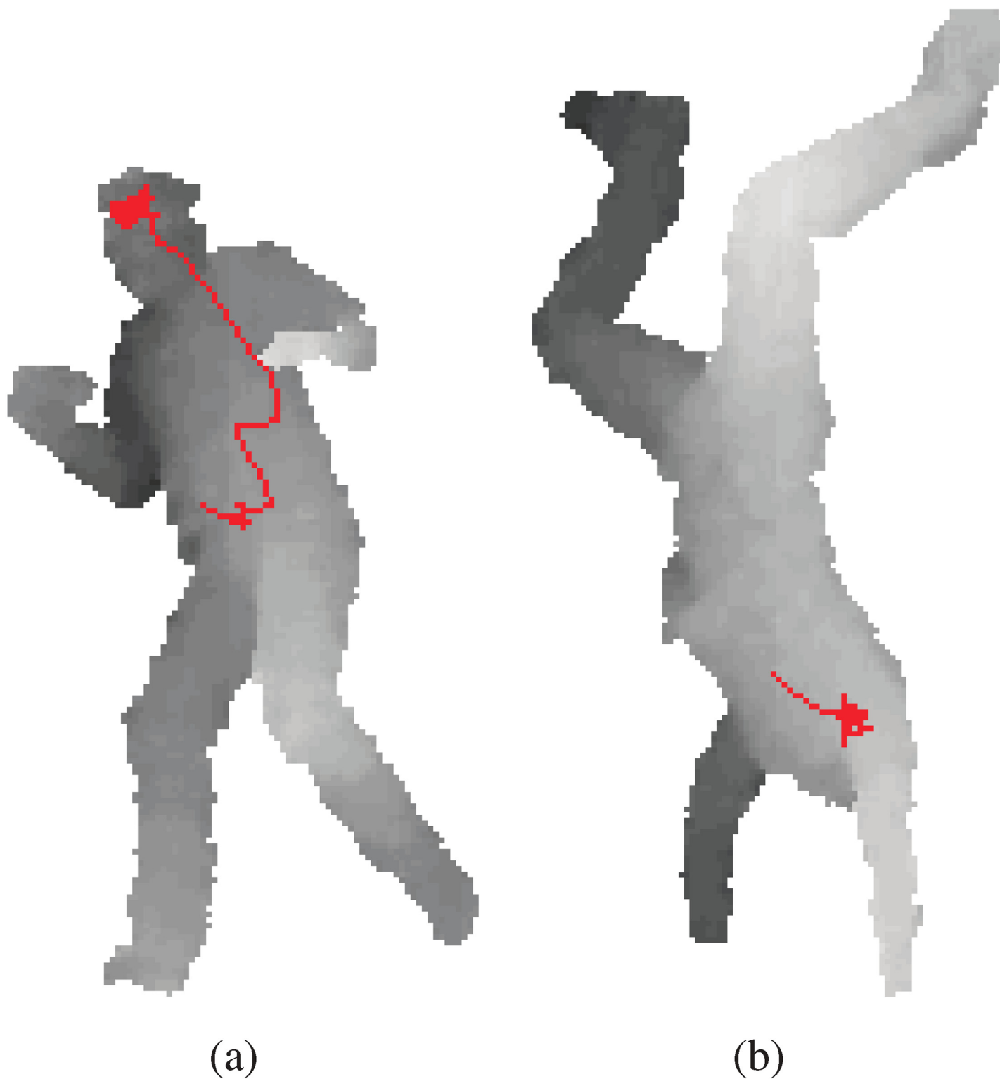
Fig 1. The red lines represent the random forest walks trained to find the position of the head. The random walk starts from the body center in (a). In (b), the head position is found with fewer steps by starting from the chest, which is much closer than the body center.
