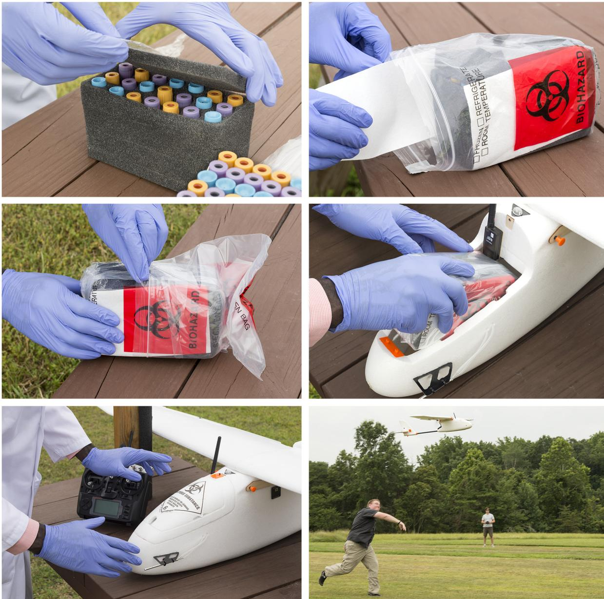
**Fig 2. Figure showing the packing of the sample payload.** 1. Custom-cut foam block. 2. Placement of sealed foam lock in the bio-hazard bags as well as absorbent material for potential sample containment. 3. Placement of first bio-hazard bag inside the second bio-hazard bag. 4. Placement of double-wrapped payload in the fuselage. 5. Covered, secured, and labeled fuselage. 6. Launch with hand toss.
