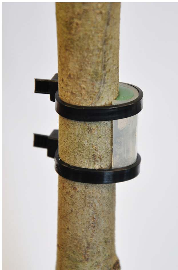
Fig 1. Chamber designed for confining adult female X. germanus and X. crassiusculus to stems of flood-stressed and non-flooded Cornus florida .
