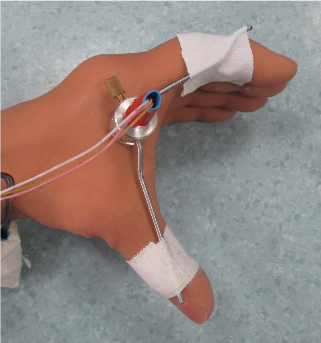
**Fig 3. Potentiometer attached to the prosthesis hand.**
