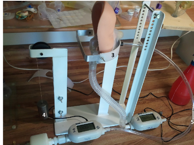
Fig 1. Test Assembly. (#1) Inflow meter represents the baseline ("complete seal") and reflects maximum available inspiratory flow. (#2) Outflow meter input port is connected through flexible tubing to the "trachea". Its exit port is open to the atmosphere. The airflow measured at this flow meter represents the flow volume through the mask and the model. (#3) Belt holding the mask to the model with various forces (#4).
