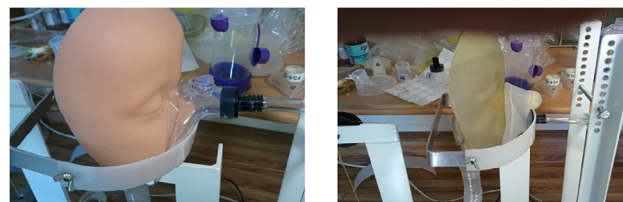
Fig 2. Faces with Masks. (A) Soft face with a SootherMask (B) Hard face with an Aerochamber mask.
