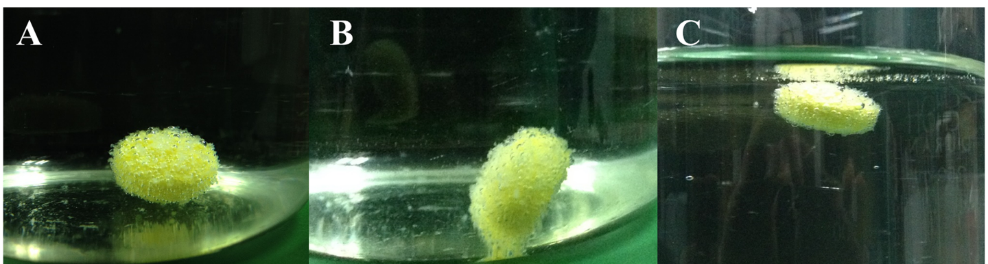
Fig 6. Enclosed effervescent system of the formulated imatinib mesylate (F6) floating sustained-release tablet with carbon dioxide-generated bubbles in 0.1N HCl, (A), after 10 s (B) and after 13 s (C) floated after 36 s.
